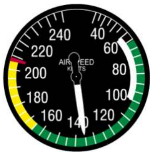
Figure 3-4.— Conventional Color-coded Airspeed indicator.
