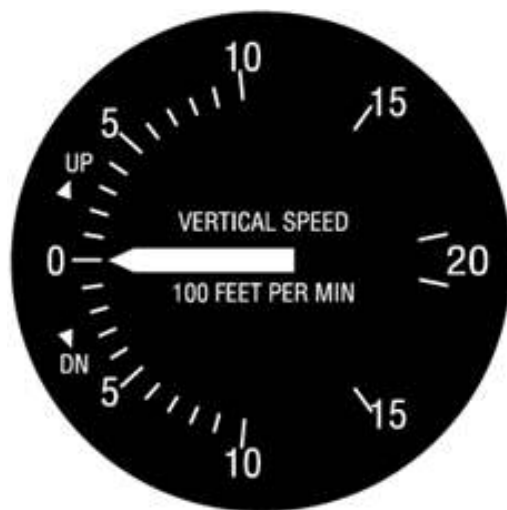
Figure 3-3.—Vertical speed indicator.
