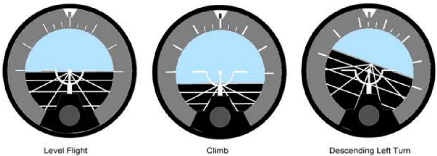
Figure 3-11.—Various indications on the attitude indicator.
