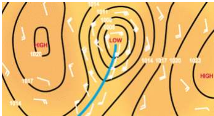
Figure 5-24.—Weather map indication of wind shift line (center line leading to low).
