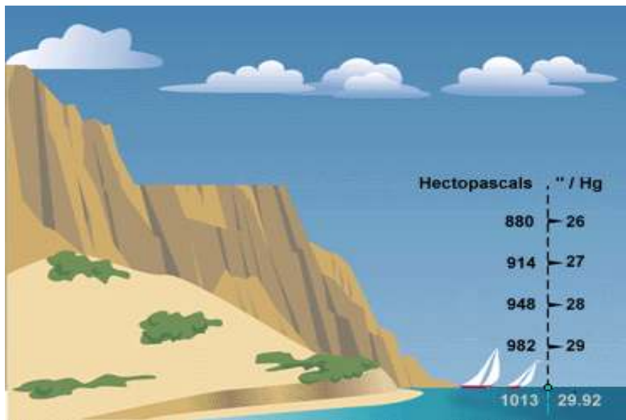
Figure 5-2.—Barometric pressure at a weather station is expressed as pressure at sea level.
