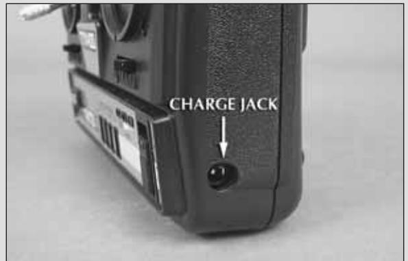
The Tactic 4-channel transmitter is equipped with a charge jack that will allow you to use a rechargeable NiCd battery pack and charge it directly through the transmitter. For a rechargeable pack that works with this transmitter, use part number FUTM1450 Transmitter NiCd 9.6V 500mAh.
