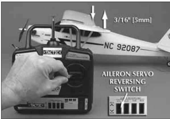
□ 3. By moving the right control stick left, the left aileron must move up and the right aileron must move down. If they do not, change the position of the aileron servo reversing switch on the transmitter. When the right stick is moved all the way to the left, the trailing edge of the left aileron at the inward side should move **up 3/16" [5mm]**. When the right side stick is moved all the way to the right, the left aileron should move **down 3/16" [5mm]**.
