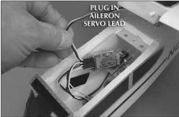
❑1. The receiver is secured to the fuselage with hook and loop material. Pull the receiver free and plug the aileron servo lead from the wing into Channel "1" with the white wire facing up (the channels are numbered on the bottom of the receiver). Push the receiver back onto the hook material.
