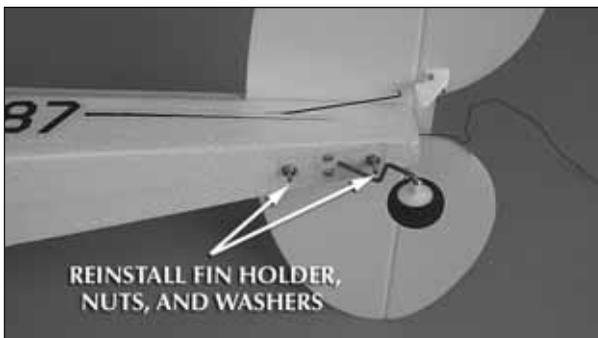
❑ 3. Reinstall the fin holder with the stabilizer onto the fuselage. Reinstall the two washers and the two nuts on the threaded rods. Use the included wrench to tighten the nuts, **being careful to not crush the foam**.
