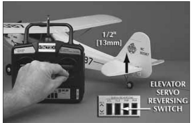
□ 2. By moving the right stick down, the elevator must move up. If it does not, change the position of the elevator servo reversing switch on the transmitter. When the right stick is moved all the way down (towards you), the trailing edge (back edge) of the elevator should move up 1/2" [13mm]. When the right stick is moved all the way up (away from you) the trailing edge of the elevator should move down 1/2" [13mm].
