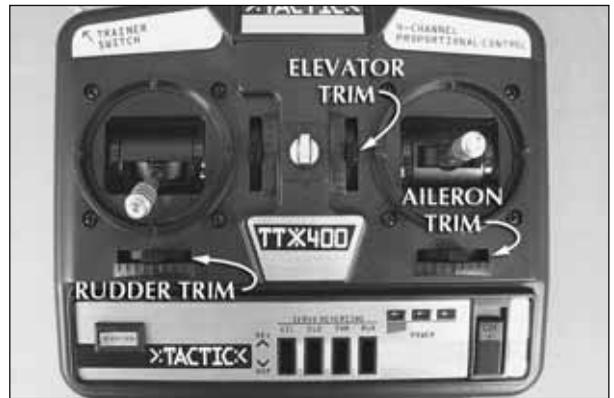
❑ 2. Center the rudder, aileron, and elevator trim.
