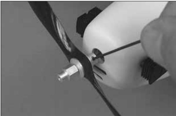
□ 4. The set screw in the prop adapter should be checked and tightened **before** each flight.
